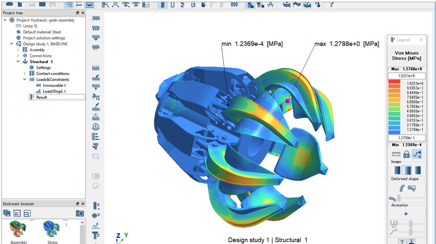
Altair SimSolid is a structural analysis software developed specifically for rapidly evolving design processes. It eliminates geometry simplification and meshing, the two most time-consuming and expertise-extensive tasks done in traditional FEA, enabling the analysis of fully-featured CAD assemblies in minutes without meshing.
